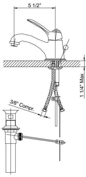
Suggested sink hole dimension is 1  $\frac{1}{2}$ " Maximum sink hole dimension is 1  $\frac{5}{8}$ " Minimum sink hole dimension is 1  $\frac{3}{8}$ "
